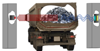
Neutron activation sensor to analyse scrap bulk composition directly in the container during delivery
