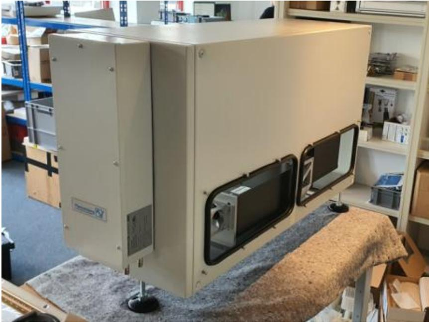
*Figure 8: Optical module of the LIBS sensor during setup at LSA premises, back view with access hatches for alignment purposes.*
