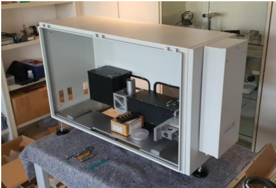
Figure 7: Optical module of the LIBS sensor during setup at LSA premises.
