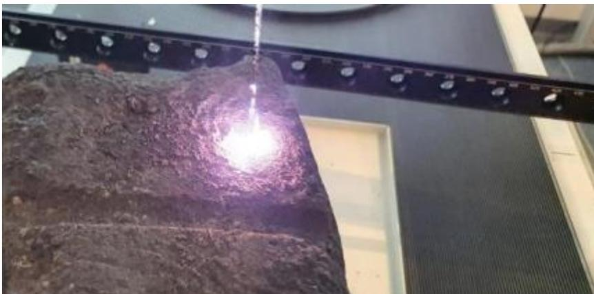
*Figure 9: Ignited plasma on a test sample, ignited with the test setup of the LIBS module.*
