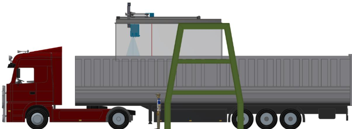
*Figure 3 Concept of installation of the LIBS sensor for material delivered and analysed on a truck.*
