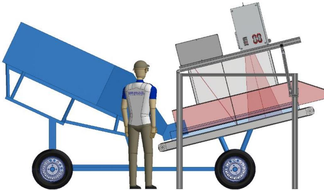
*Figure 2 Concept of installation of the LIBS sensor at a conveyor belt material flow.*
