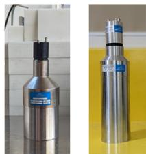
Fig. 3. Photo of one of the LaBr3 detectors (a) and BGO (b) used in the experiments.
