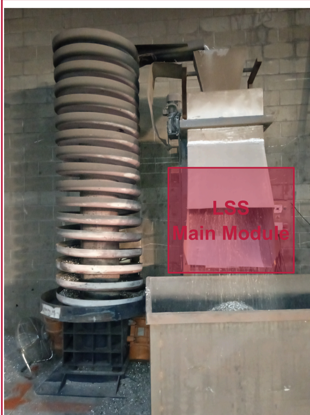
Fig. 1: The real industrial conditions at Grupal-Art plant - the cleaned aluminum chips are elevated and dropped into a container. The red area shows the place for the LSS introduction.
