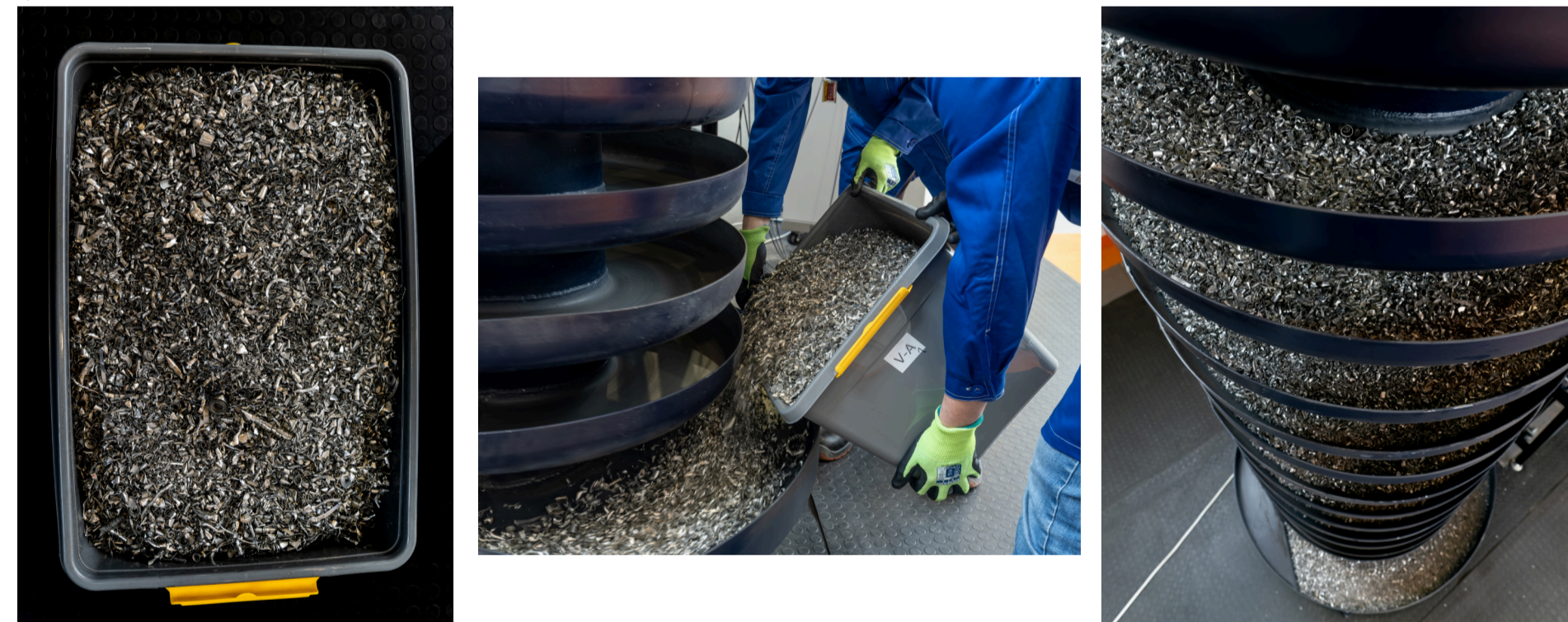
Fig. 4: Photos of industrial samples of aluminum chips provided by Grupal-Art for industrial tests of the LSS demonstrator.
