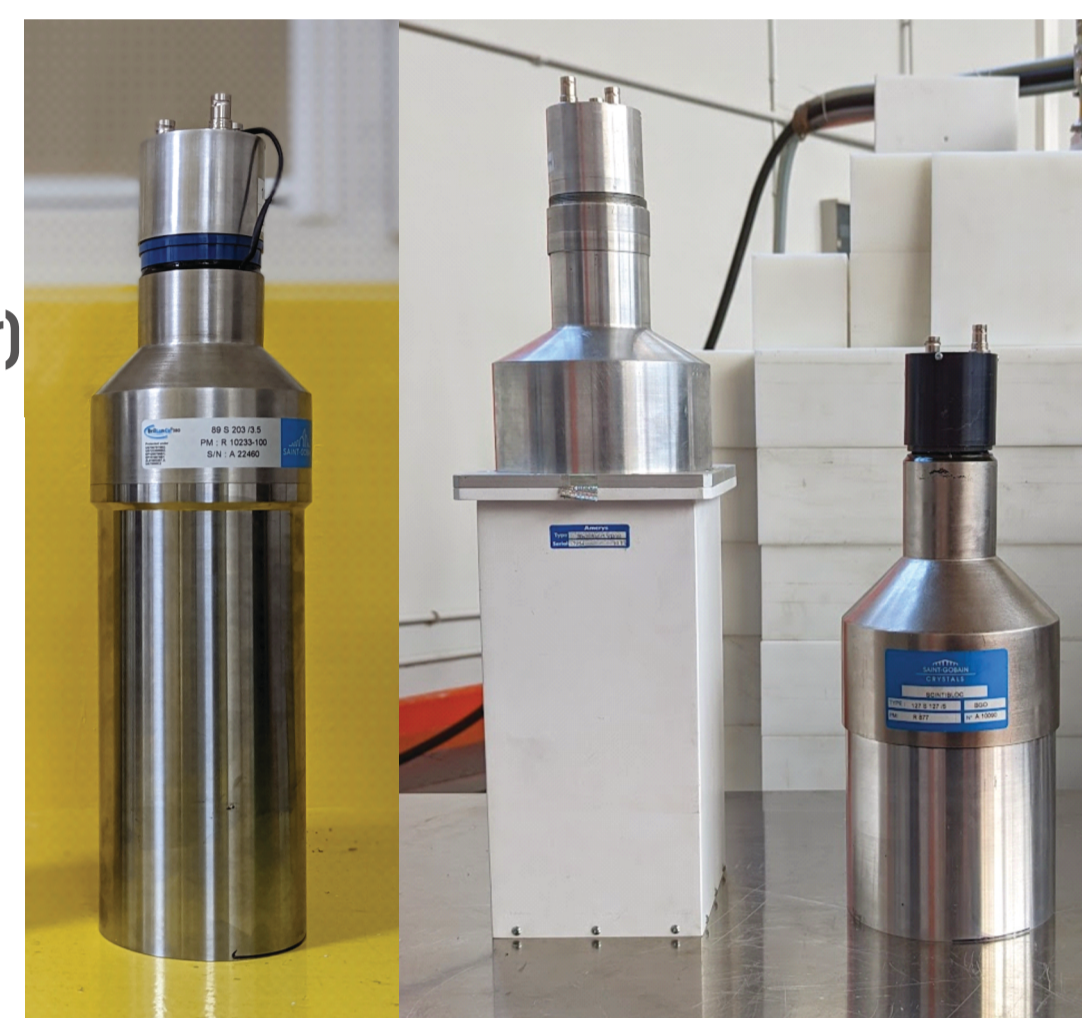
Fig. 3: One of the possible layouts of scintillation detectors inside the LSS Main Module (left) and photos of the detectors possible for application inside the LSS: LaBr 3 , NaI, BGO (starting from right).
