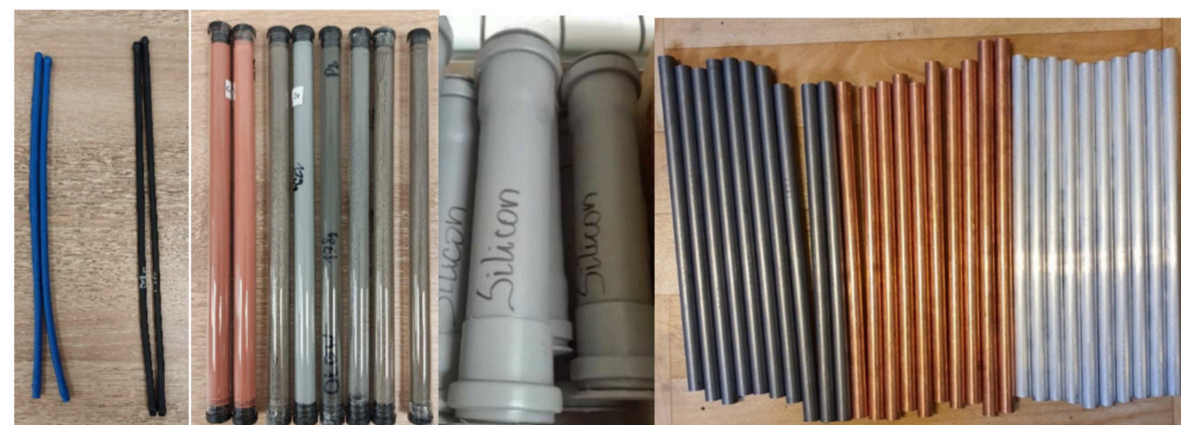
Fig. 5: The pure element samples prepared for calibration of the LSS prototype: a) plastic packets 200-250mm long and 4-5mm in diameter, b) plastic pipes 250mm long and 12mm in diameter, c) plastic rods 250mm long and 45mm in diameter, d) metal (Fe, Cu, Al) rods 250mm long and 12mm in diameter.
