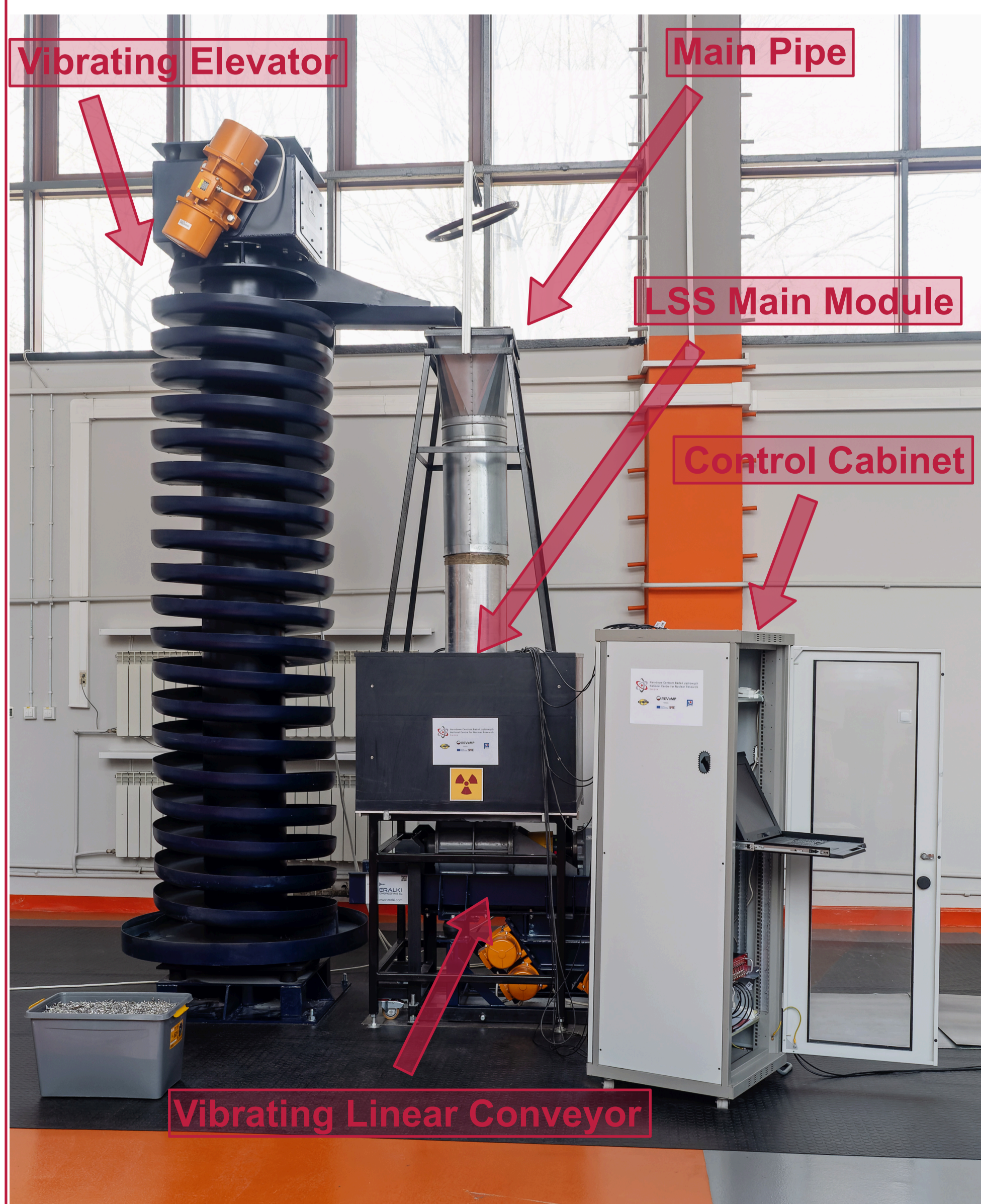
Fig. 2: Photo of the LSS demonstrator placed in the experimental setup that mimics the industrial conditions at Grupal-Art aluminum refinery.
