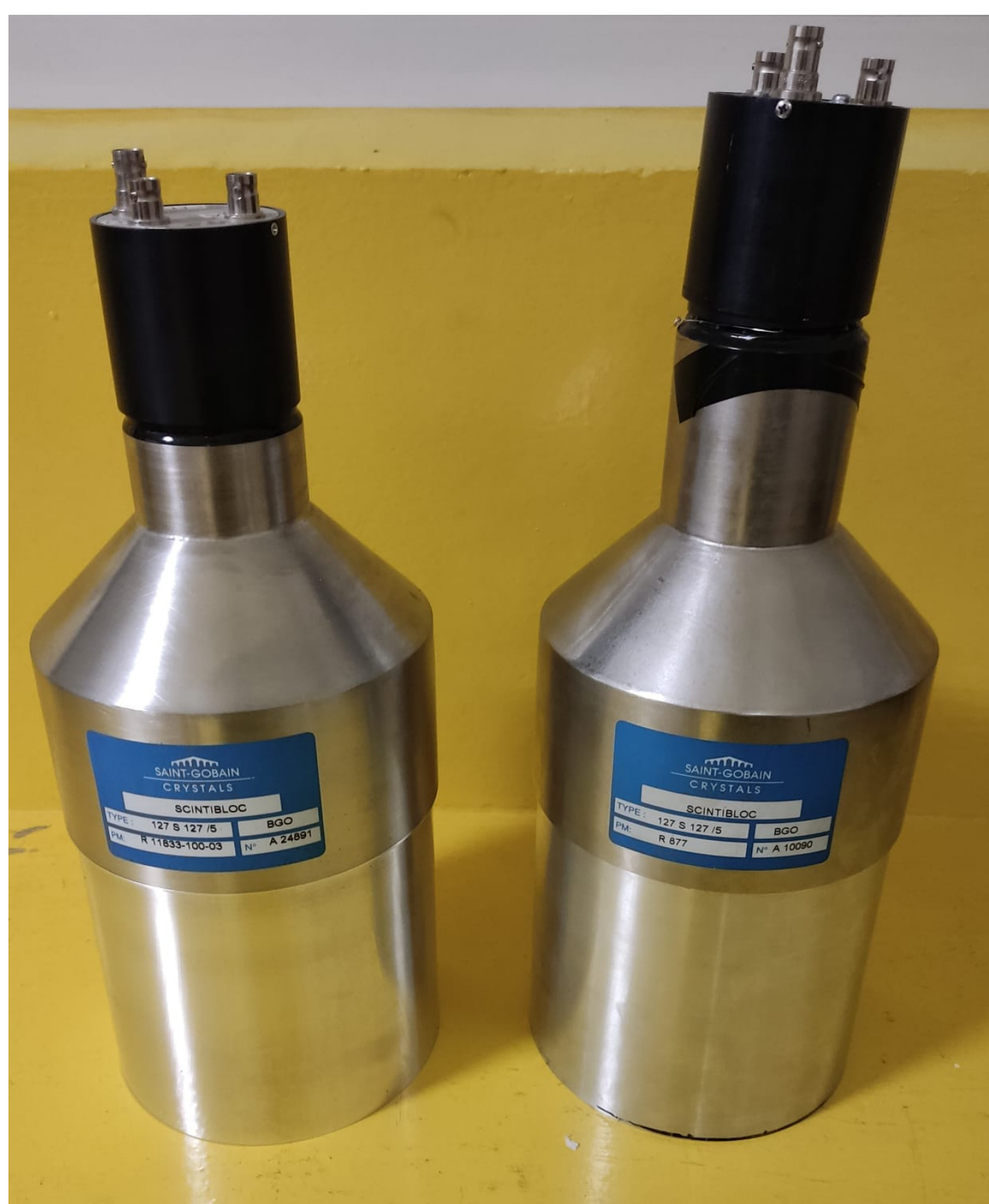
Fig. 1. Detectors used in the experiment, from the left: 5x5inch BGO coupled to the R11833-100 and 5x5inch BGO coupled to the R877.
